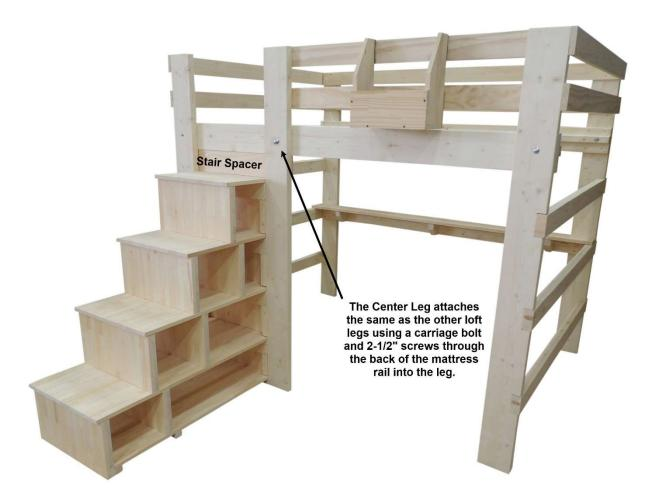
Once the frame is set up, the center leg can be attached to the bed. There is only 1 center leg which is attached to the front rail. The leg will have a hole drilled for a carriage bolt and will be labeled as the center leg. Find the predrilled hole in the front rail and attach the center leg a using 5" carriage bolt. Hand tighten the carriage bolt to hold the center leg in place but do not add the 2-1/2" screws around the carriage bolt.
